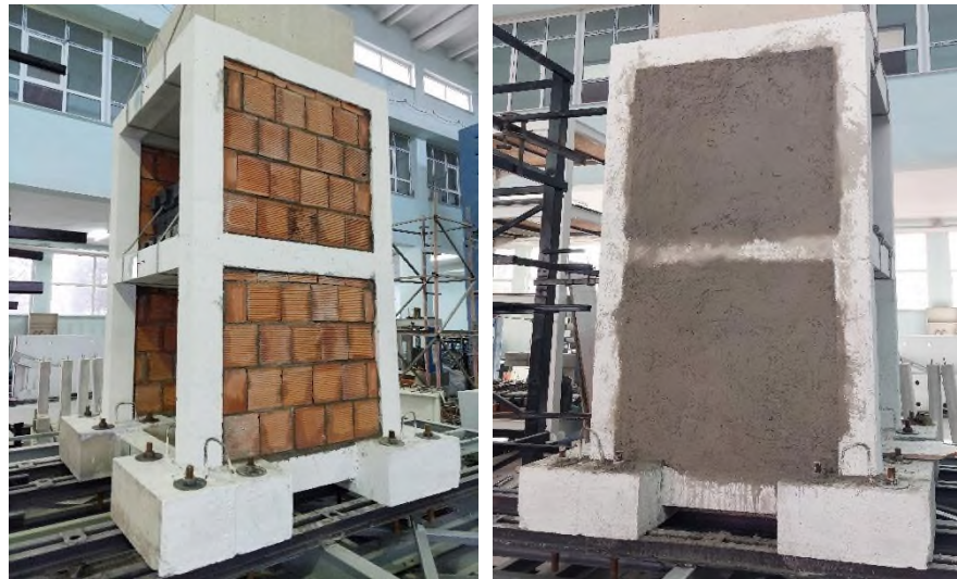
Figure 12. Improvement with infill walls
