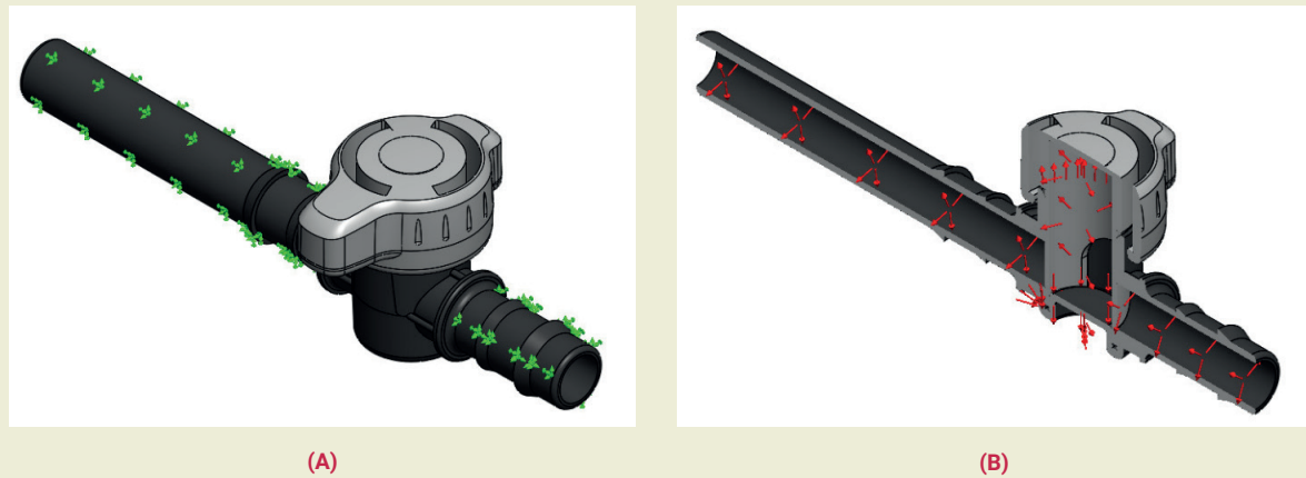
Figure 3. Boundary conditions of the analyzed mini valve A) fixing surfaces and B) pressure application surfaces
