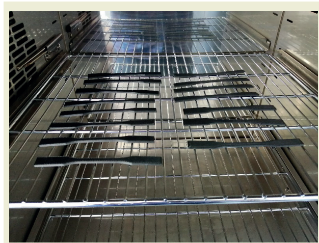
Figure 2. Annealing of the tensile test specimens in the oven
