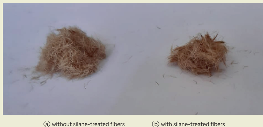
Figure 2. Jute fibers with and without silane-treated fibers.
