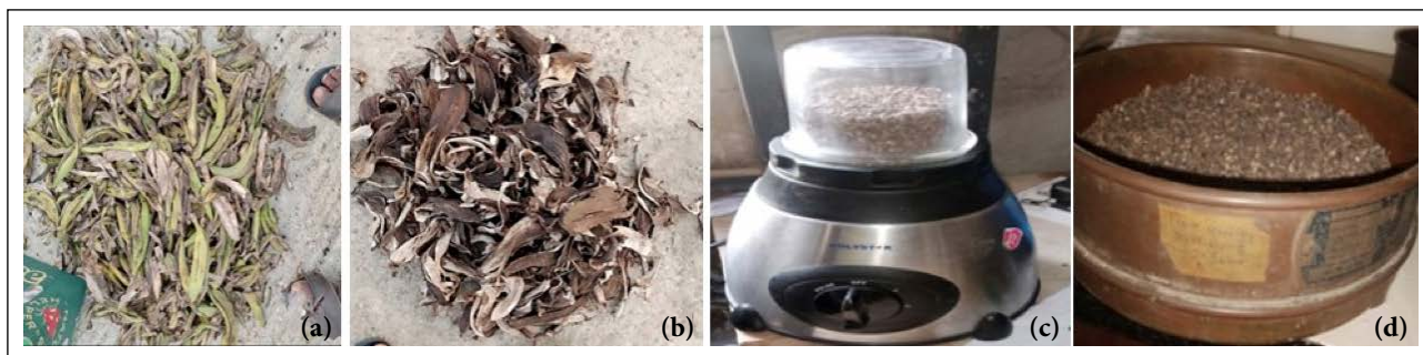
Figure 3. Preparation of UPP sample (a) UPP as collected, (b) sundried UPP, (c) grinding process, (d) sieving of UPP sample.
