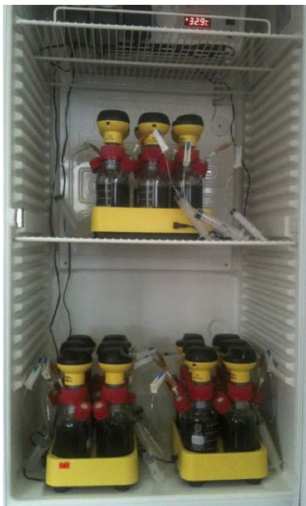
Figure 2. Batch reactor (Oxiotop C bottles).
