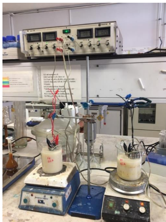
Figure 1. Electrocoagulation Experimental Set-Up
