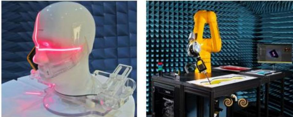
**Figure 3.** An overview of SAR measurement setup
