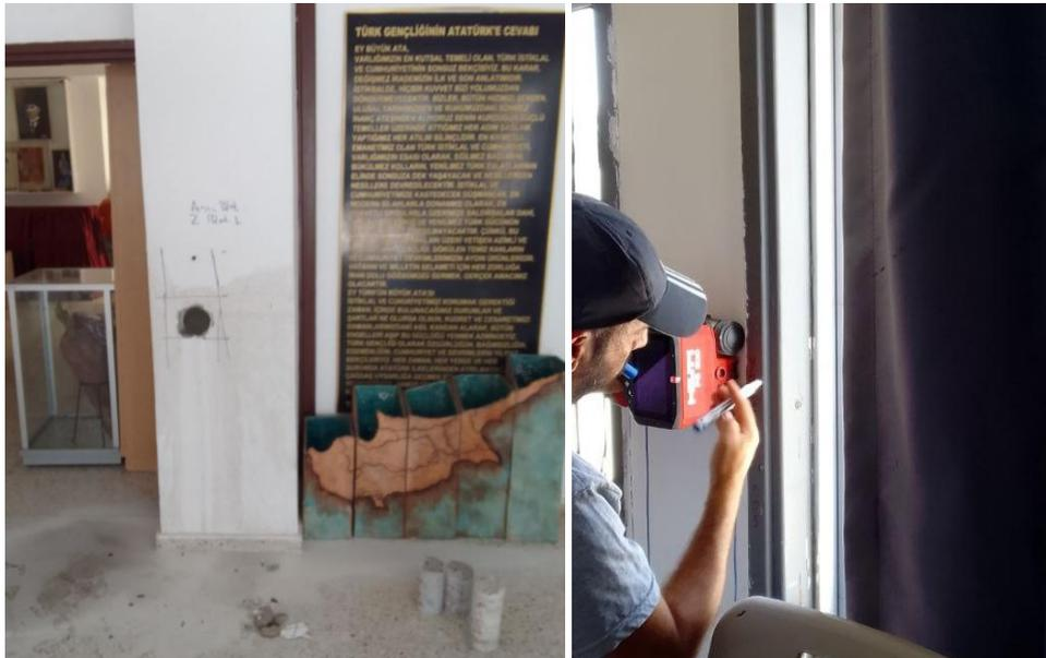
**Figure 3.** Laboratory test for validation; a) Extracted concrete cores for compression test; b) Scanning concrete rebars
