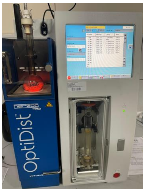
Figure 2. Determination of distillation temperatures of test fuels
