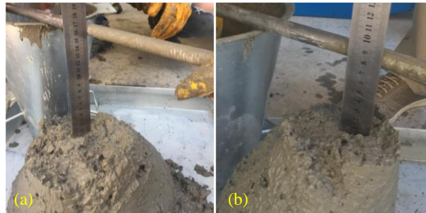
Figure 5. Slump values of (a) PL; (b) PSA10.
