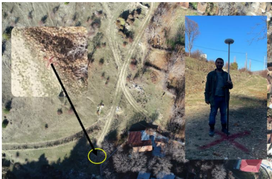
Figure 3. GCP marking and GNSS-CORS device measurement pictures on the study area
