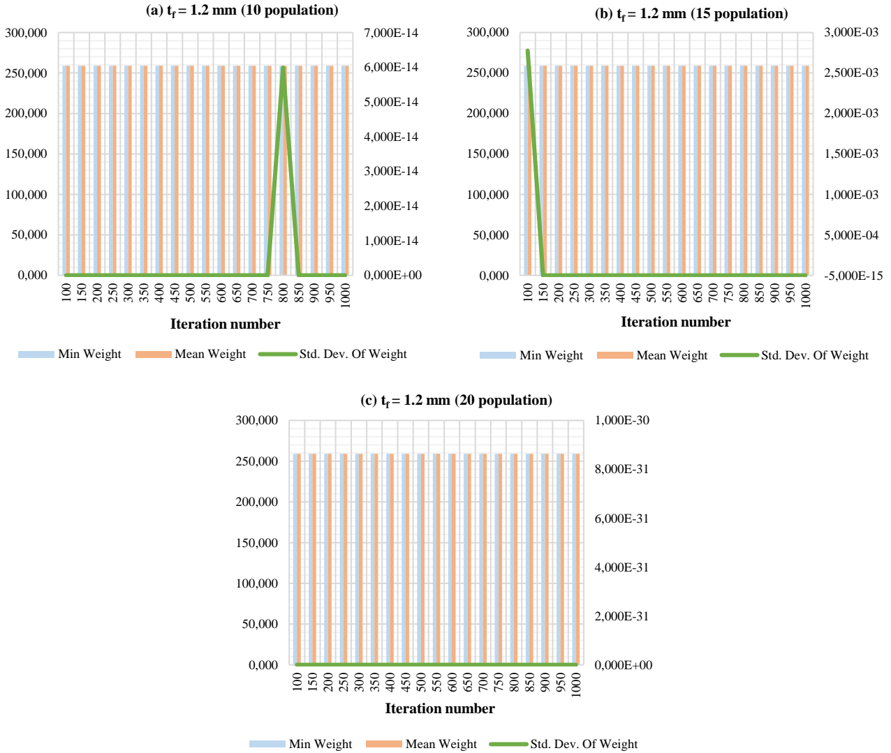
Figure 2. Distribution of min, mean and standard deviation of weight values according to iterations (FPA).
