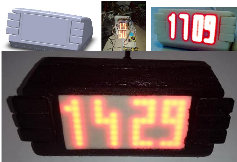
Figure 1. CAD rendering and the prototypes of a table clock product concept (designed and built by the author).
