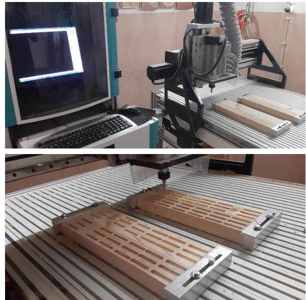
Figure 6. CNC machining of specimens
