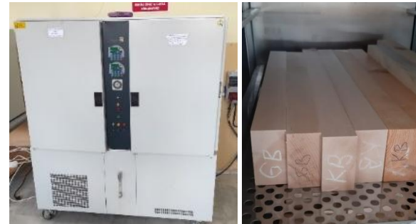
Figure 3. Keeping the specimens in the air conditioning cabinet
