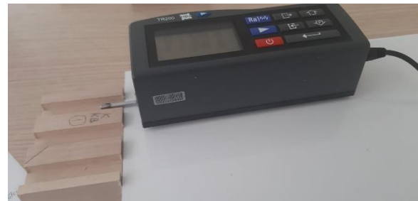
Figure 7. Roughness measurement of specimens
