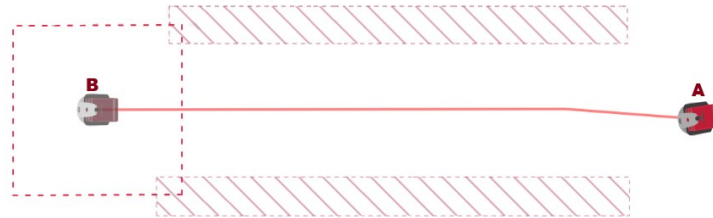
Figure 19. In an empty aisle, with the RT detection model deactivated, the process of the PIXER robot planning its route globally and initiating movement locally.
