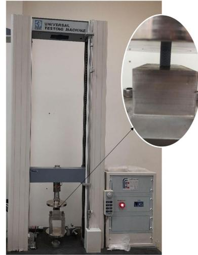
**Figure 5.** Demonstration of the Gotech universal testing machine utilized for conducting the simple compression tests.
