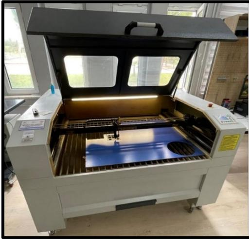
**Figure 2.** CO<sub>2</sub> laser cutting device.
