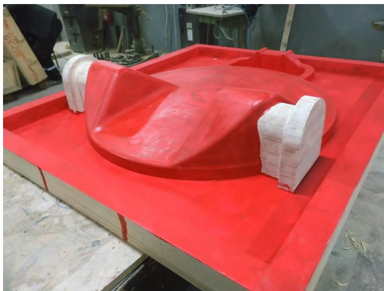
Figure 12. The finish pattern of the ring for the body assembling
