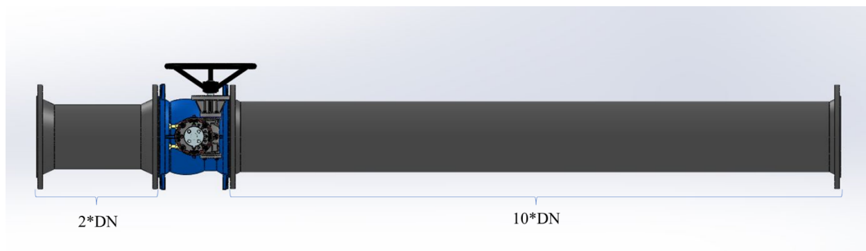
Figure 15. Three-dimensional valve test verification model
