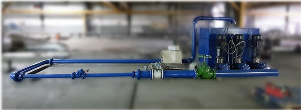
Figure 17. Kv test setup for the designed prototype
