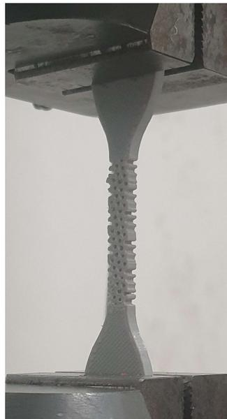
Figure 6. A specimen of the tensile test.
