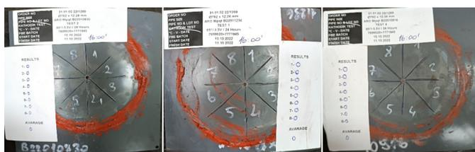
Figure 8: Cathodic peeling test samples
