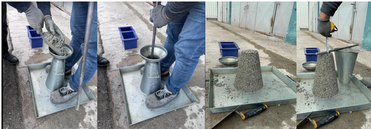
Figure 2. Applied Slump Test
