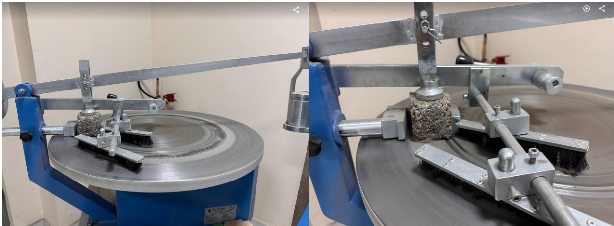
Figure 3. Abrasion Application to The Sample
