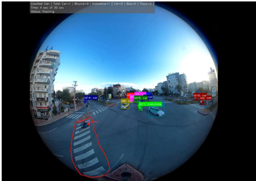
Figure 11. Video output of vehicle tracking, classification, and counting visualization
