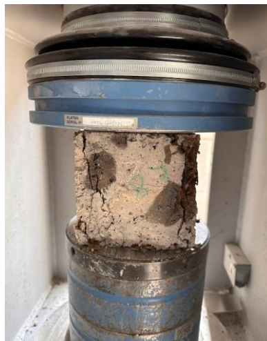
Figure 5. Applying Compressive Strength Test to Concrete
