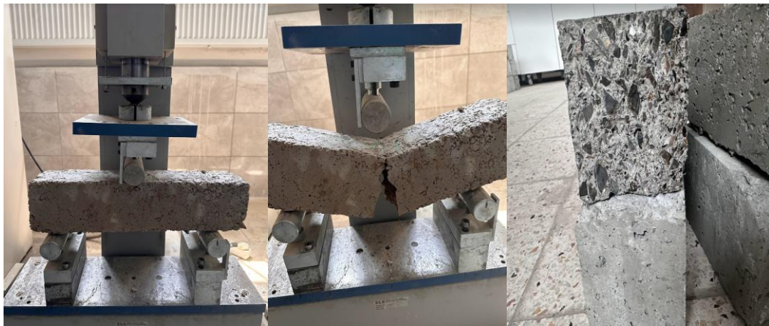
Figure 6. 3-Point Flexural Strength Test Application
