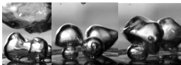
Figure 13. Events of bubbles merging in the vicinity of the boiling surface in horizontal, vertical, and diagonal axes [28].
