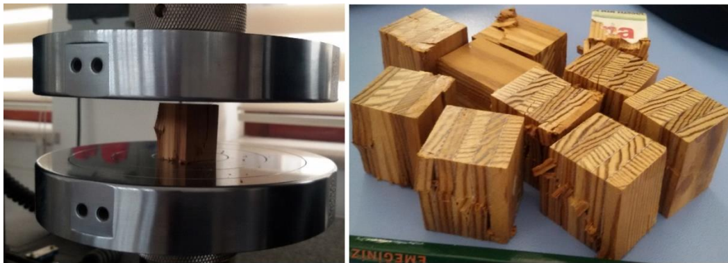
Figure 3. Compressive strength parallel to the grain test setup and test samples
