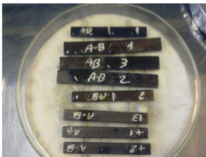
Figure 1. A typically of several BA-T-WPC and BA-PT-WPC samples exposed to white-rot fungus using the agar-block test method
