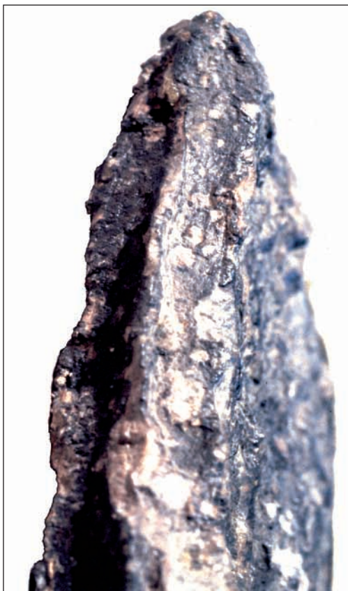
Fig. 9. Edge of quarter oxide ingot KW 204 showing evidence of cutting from both sides with a chisel and then breaking the portion of bridging metal in the middle by repeated bending of the ingot in opposite directions.
