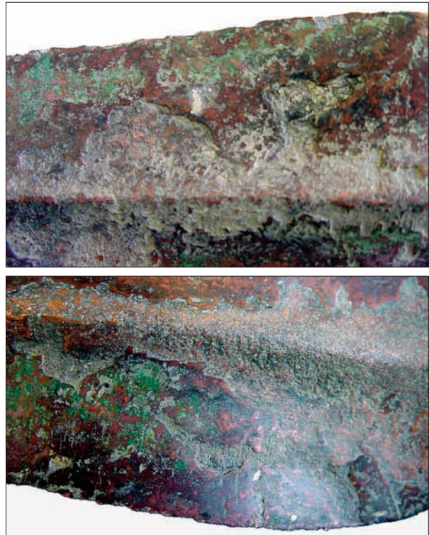
Fig. 6: Relics of tin (white) on the former spearhead surfaces released from the corrosion
