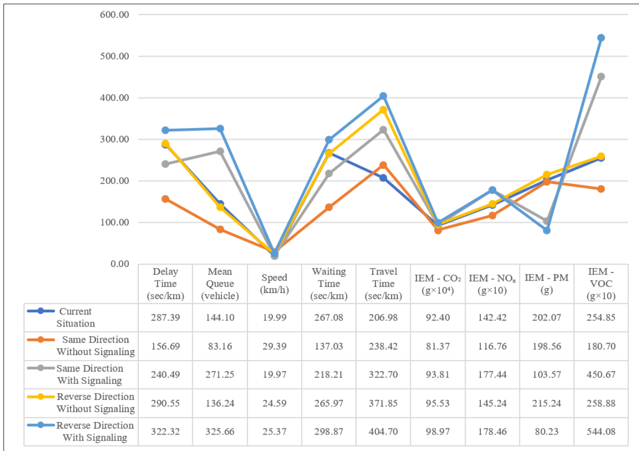
Figure 13. Comparison of the simulation findings between five scenarios using analysed metrics (IEM means Instantaneous Emission Model)
