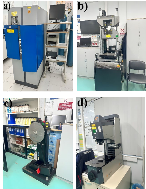
Figure 5. Devices used for testing welded samples, spectrometer instrument (a), tensile tester (b), notched impact tester (c), hardness tester (d)
