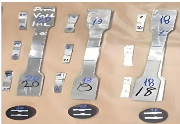
Figure 4. Tensile test, notch impact test and microstructure test samples a) 5 l/min (19), b) 12 l/min (18), c) 20 l/min (20)
