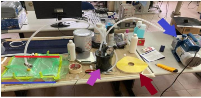
Fig. 6. A normal setup for the resin infusion process
