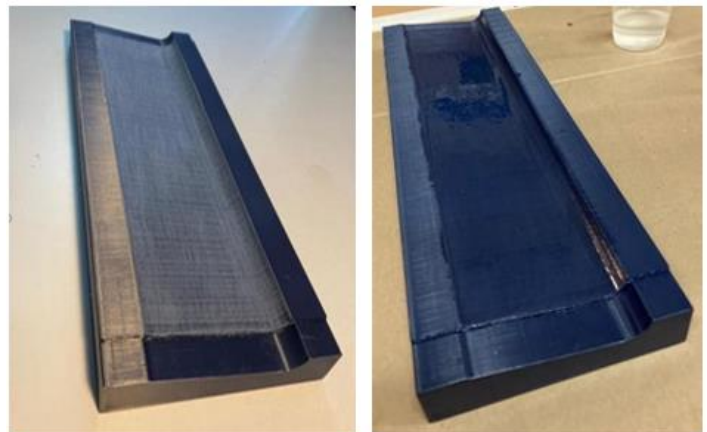
Fig. 14. Rudder mold: (a)After sanding. (b)After gelcoat
