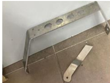
Fig. 17. Landing gear. Version-1 (left). Version-2 (middle), Installed landing gear (right)
