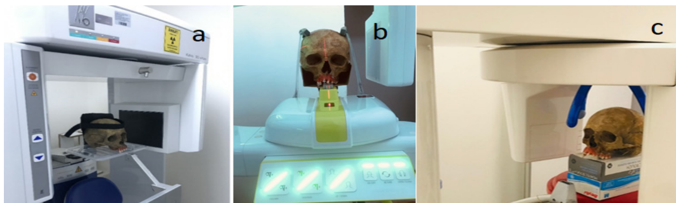
Figure 2. Images taken while scanning on different brands of CBCT devices; (a) KaVo 3D eXam, (b) Rainbow CT, (c) Orthophos XG 3D.
