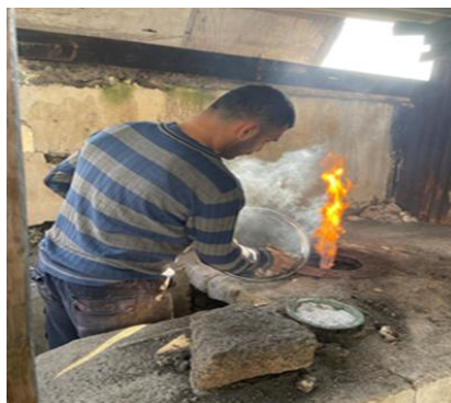
Image 14: Sprinkling Ammonium Chloride on the Copper Tray
