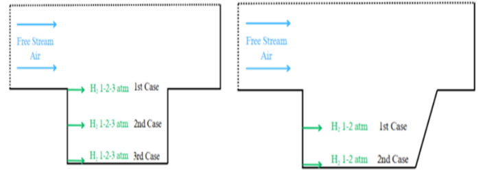
Fig.8. Rectangular and trapezoidal cavity configuration
