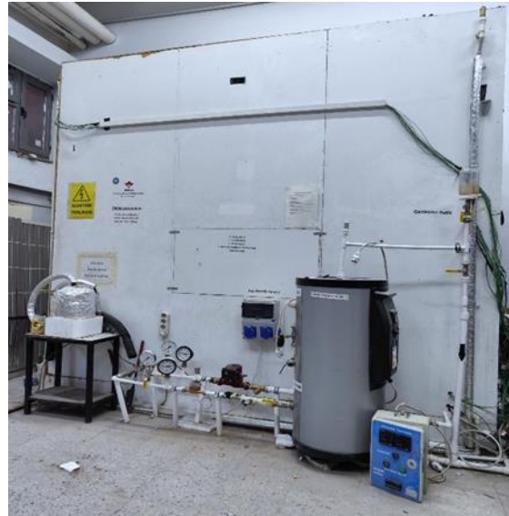
Figure 5. View of the radiator test measurement set-up
