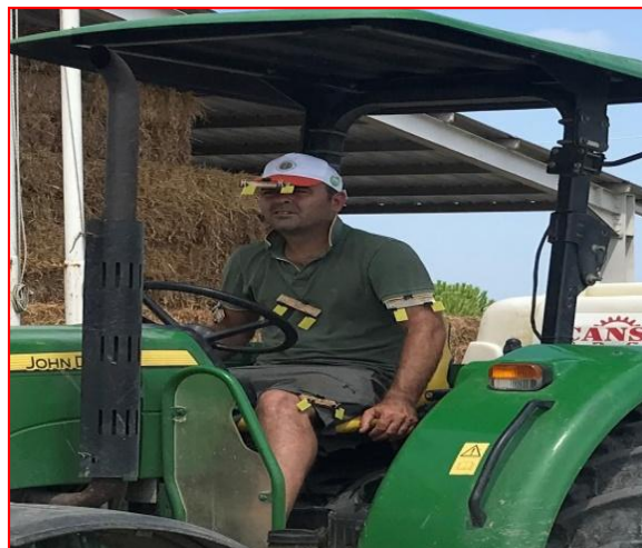
Figure 5. The positioning of WSP on the operator.
