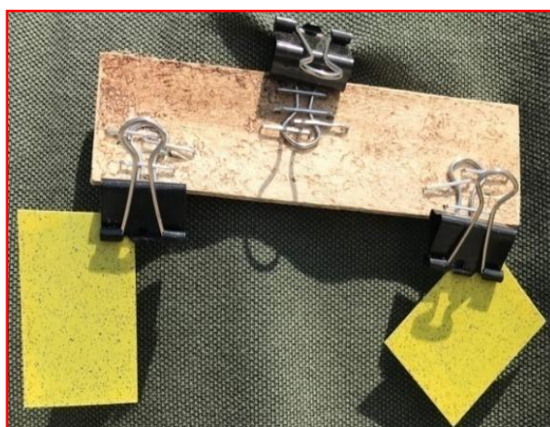
Figure 2. Clamp for water sensitive paper attached to the operator.
