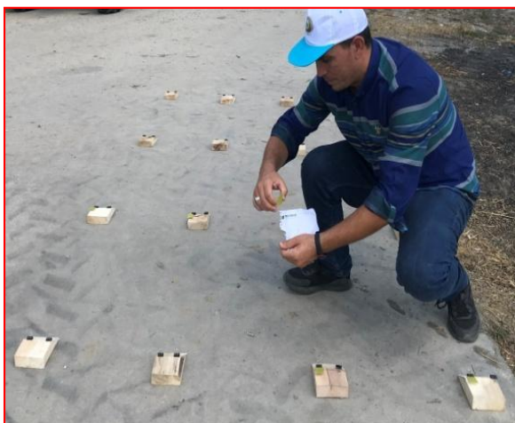
Figure 4. Placement of water sensitive papers (WSP) on blocks in the experimental area.
