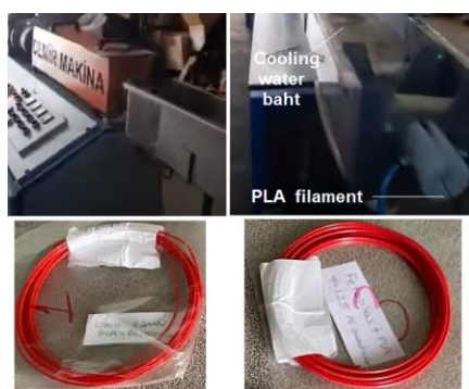
Figure 1. The production process and PLA filaments obtained.
