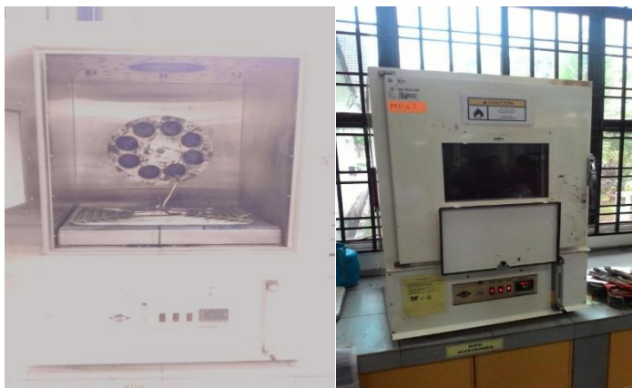
Figure 9. Rolling Thin Film Oven Test ( RTFOT) machine
