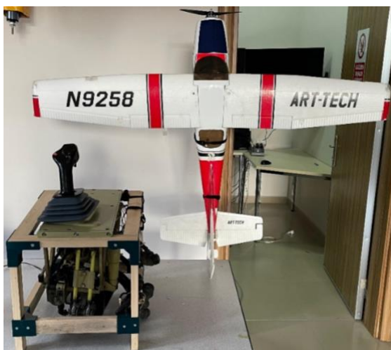
Figure 2. Integration of A320 Side-Stick Controller with UAV via Electronic Control Unit
