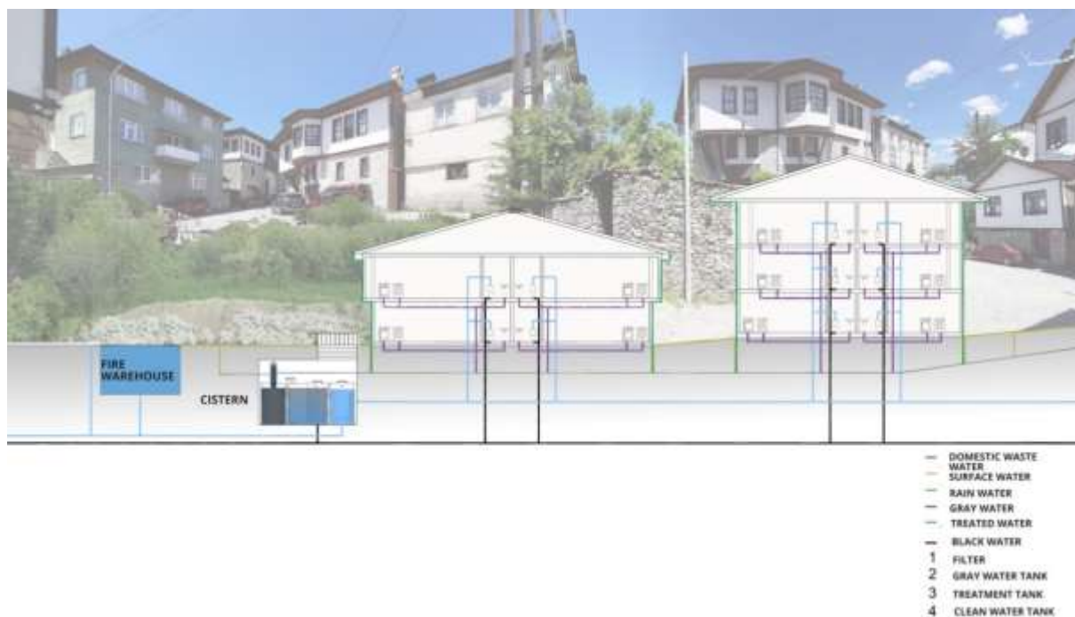
Figure 7. Section Diagram of Proposed Theoretic Greywater Treatment System
