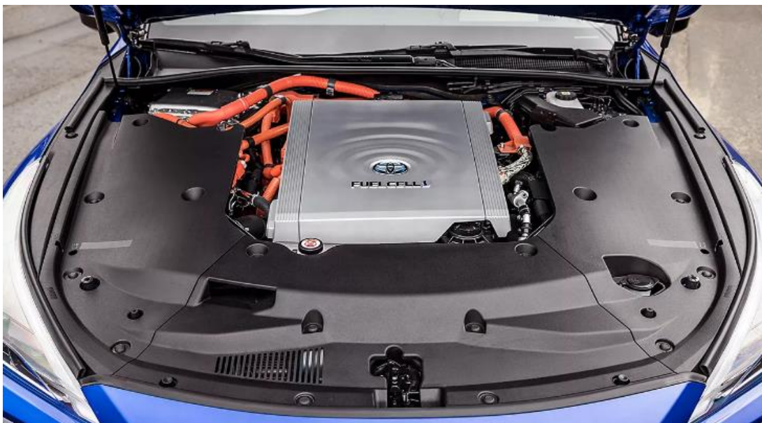
Figure 6. Actual image of the fuel cell in the Toyota Mirai vehicle
