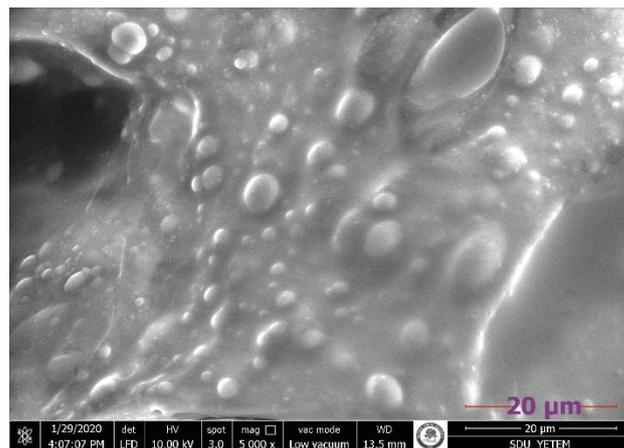
Figure 4 SEM images of microencapsulated vitamin E
