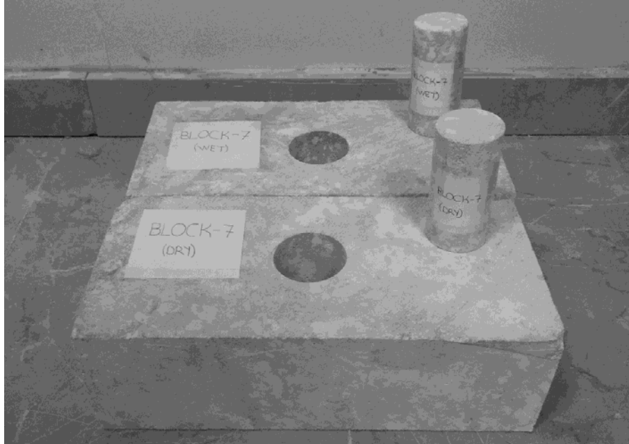
Figure 1 - Adjacent parts of Block-7 and NX size samples taken from the middle
