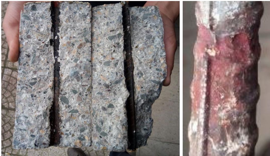
Fig. 9. the adherence state (a) of specimen-6 and the mass loss (b) of the uncoated specimen.
