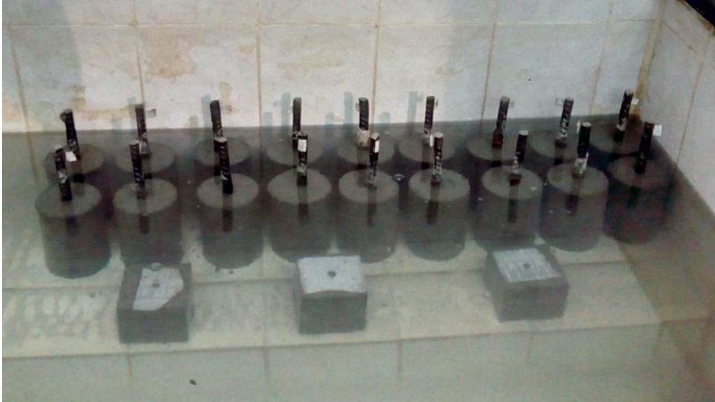
Fig. 3. Curing process of specimens.
