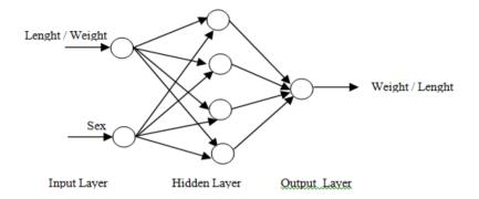
Figure 3. The ANN consisted of an input layer with 2 nodes, hidden layer, and an output layer with 1 node to be predicted for crayfish
