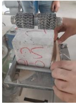
Picture 4. Abrasion Test Aparatus
