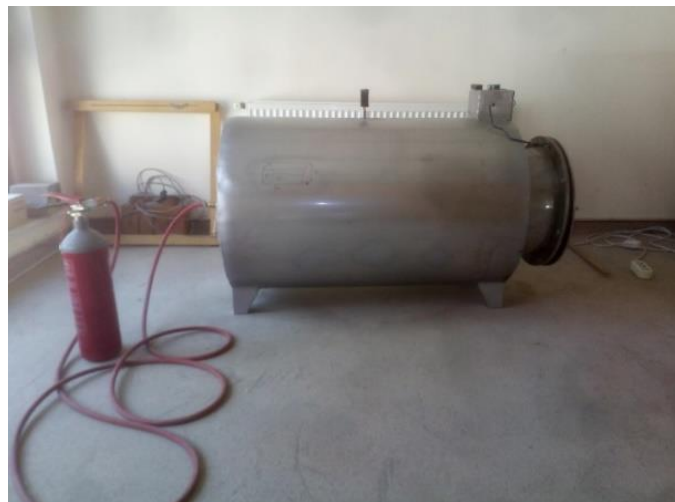
Picture 7 Carbonation test apparatus
