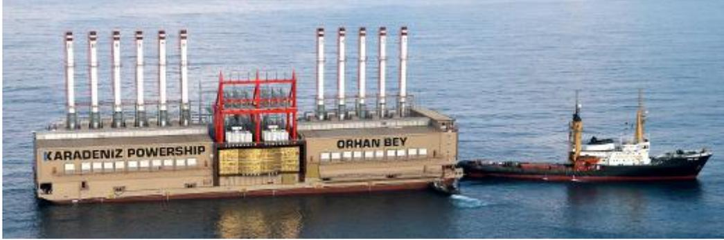
**Figure 2.** None propelled power plant
