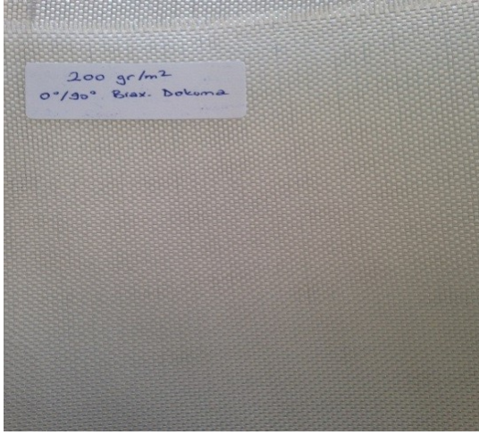
Şekil 5. 0°/90° Biaxial Cam Elyaf, 200 gr/m 2 .
