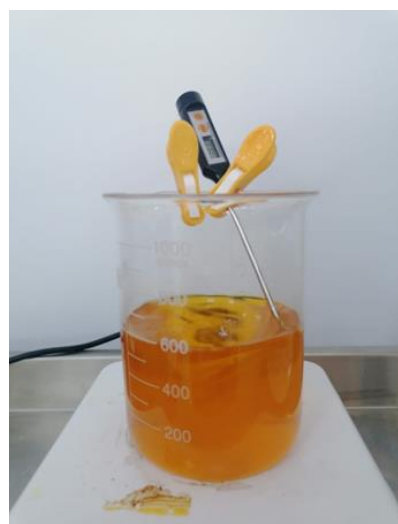
Fig. 5. Separation of water remaining in biodiesel
