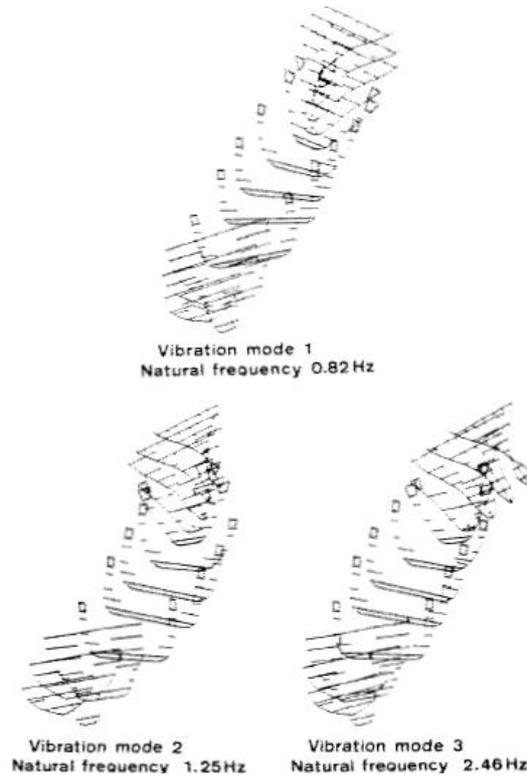
**Figure 8.** The three lowest natural vibration modes corresponding to horizontal bending-torsion models for a container ship [Pedersen (1983)]
