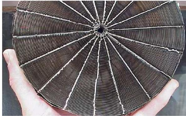
**Figure 7:** A stack made of steel with 0.4 mm distance between the plates[21]
