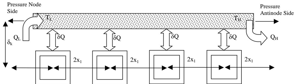
**Figure 6 :** The transfer of heat on the stack plates from one side to the other.
