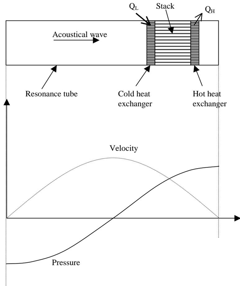
**Figure 4 :** Velocity and pressure distributions inside a simple system
