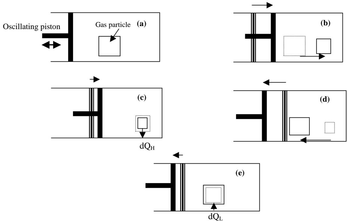
**Figure 3 :** Thermoacoustic effect in an oscillating piston-cylinder system
