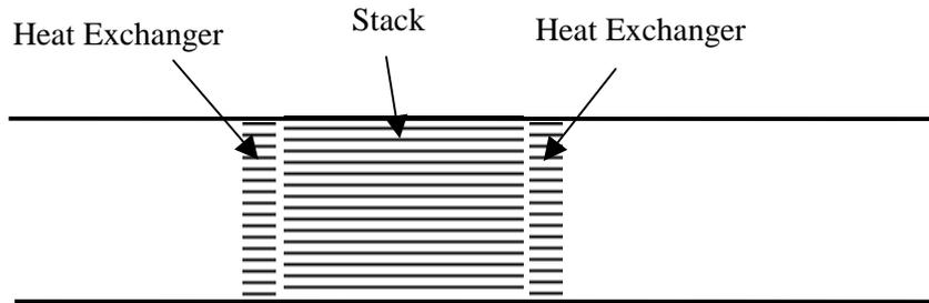
**Figure 8 :** The positions of stack and heat exchangers
