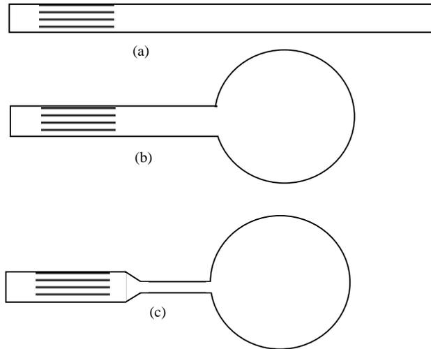
**Figure 10 :** Some types of resonance tubes
