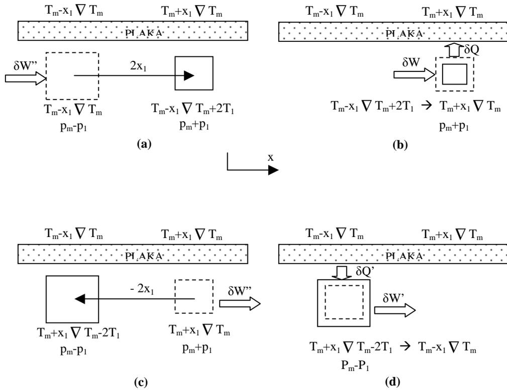
**Figure 5 :** Temperature and pressure oscillations of a particle inside a heat pump [19]
