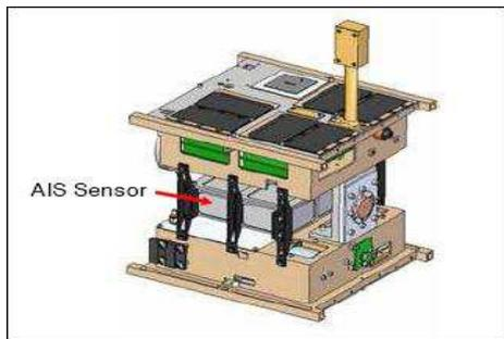
*Figure 4: Internal structure of AISSat-1 (Courtesy AISSat)*
