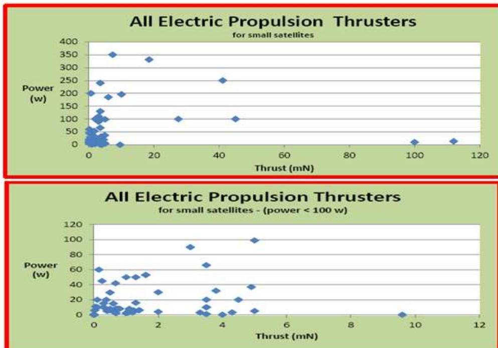
Figure 9: State of the art review of all electric propulsion thrusters available today. Results of the above mentioned graphs are being reported for thrusters available for small satellite buses (upper graph). On the below graph there is a more clear depiction of the available small satellite thrusters with power levels less than 100 W and thrust lower of 10 mN. These figures indicate solutions that can be applied (under certain circumstances) to micro and pico satellite solutions.
