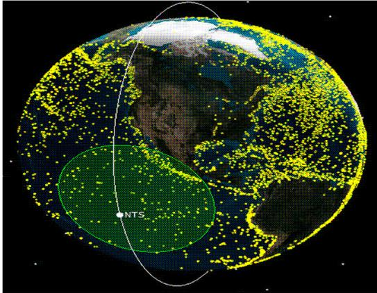
*Figure 1: Illustration of the AIS messages recovered during the first six months of NTS operations. The high density of ships in the coastal regions can be seen clearly, as can the global shipping lanes. The footprint of the NTS satellite is also illustrated, showing the large area within the footprint of the AIS receiver at any instant of time.(Courtesy: UTIAS[3])*
