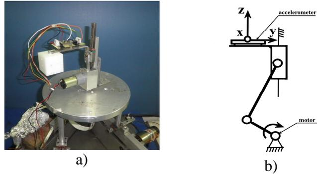
Figure 8. A test-bed slider-crank mechanism at LARM: a) an experimental set up with accelerometer and weight on the slider. b) sensing axes of the accelerometer.
