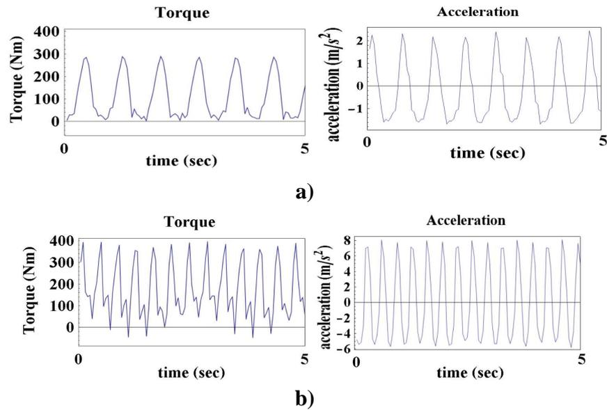
*Figure 11. An experimental measure of slider crank with servo motor without earthquake effect: a) torque data of the motor, acceleration of the slider with crank rotation 90 rpm, b) torque data of the motor, acceleration of the slider with crank rotation 180rpm*
