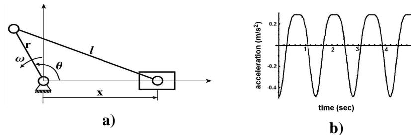
*Figure 2. A test-bed slider-crank mechanism: a) Kinematic parameters, b) Slider accelerations with stationary frame (43 rpm)*
