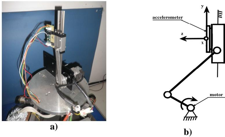
Figure 10. Slider-crank mechanism with servo motor at LARM: a) an experimental set up with accelerometer on the slider. b) sensing axes of the accelerometer.
