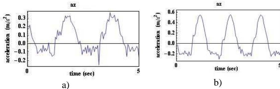
Figure 9. An experimental measure of the typical acc. of the slider-crank with stationary frame: a) crank rotation 32 rpm, b) crank rotation 43 rpm,
