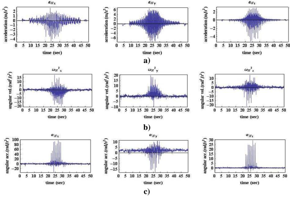
Figure 7. An example of acc. data during earthquake simulation: a) for platform center  $H$ , b) angular platform velocity, c) angular platform acc.
