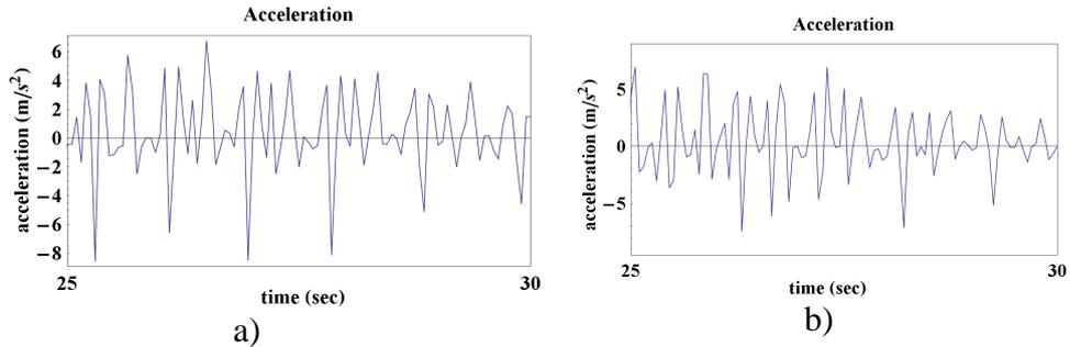
Figure 12. An experimental measure of the typical accelerations with horizontal slider under earthquake effect (type 1): a) crank rotation 32 rpm, b) crank rotation 43 rpm.
