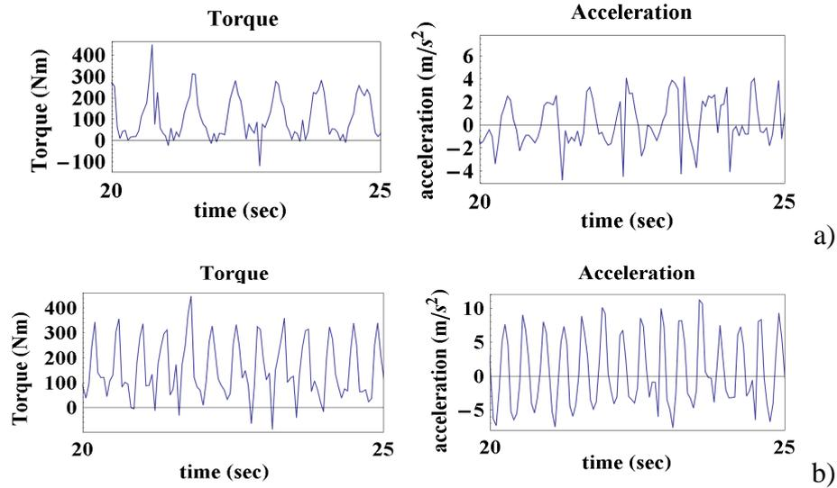
Figure 14. A measure of slider crank with servo motor with earthquake effect (type 1), torque data of the motor, acceleration of the slider with crank rotation: a) 90 rpm, b) 180 rpm
