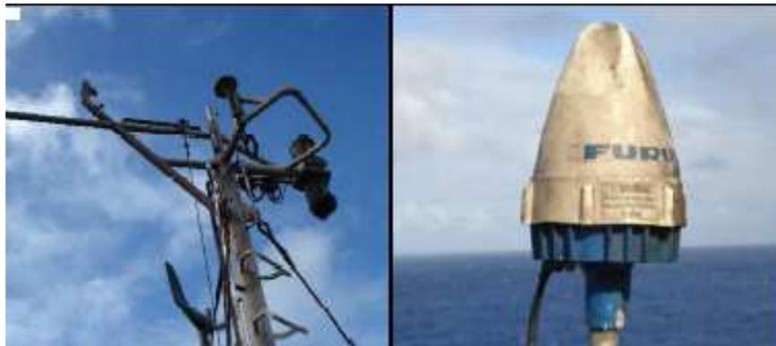
Figure 1: Electronic equipments damaged by exhaust gases.
