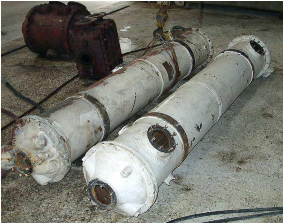
Figure 1. Seawater cooled shell and tube heat exchangers [2]
