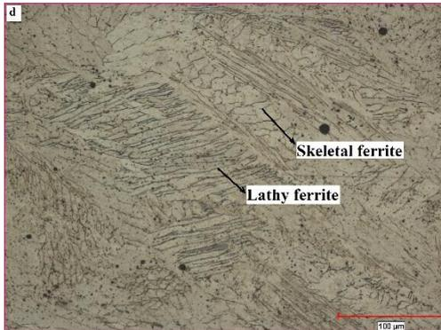
**Figure 7.** The fusion zone microstructures in high magnifications of (a) Type 8, (b) Type 4, (c) Type 1 and (d) Type 5
