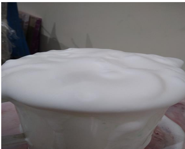
Fig. 4. Foam with homogeneous foam bubbles
