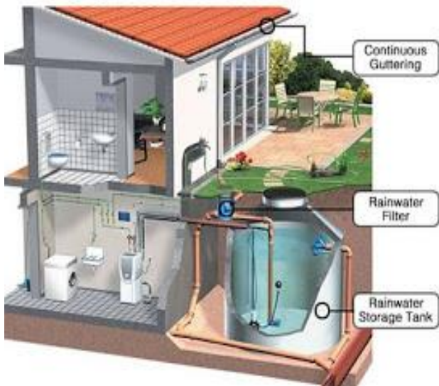
Fig.7 Rainfall Collection System
