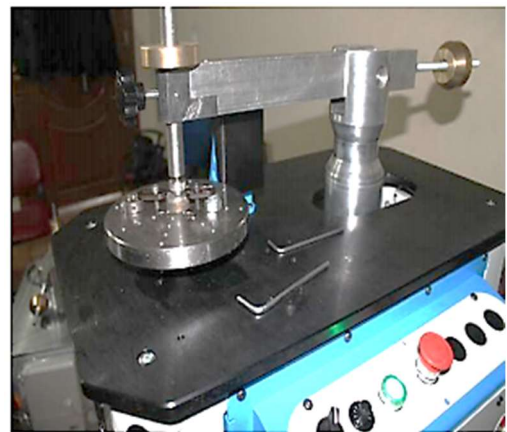
Figure 1a Experimental image of the wear test rig
